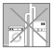
Note that to avoid condensation problems, it is essential that the dryer be fitted with the flexible hose to carry its "exhaust" at least beyond the kitchen units; preferably outside the kitchen. In order to prevent the appliance from overheating, it is important that the steam exhaust is unobstructed. Therefore, in case of a permanent hose fitted to an exterior wall or ceiling, it must be ensured an exhaust capacity of at least  $150 \text{ m}^3/\text{h}$ .
